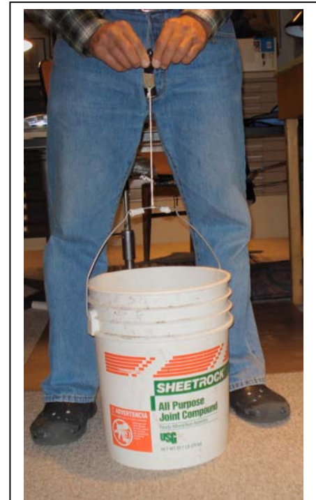
Figure 15 Measuring Separation Force between Point and Foreshaft
